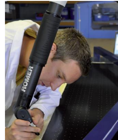
Quality Control of Photovoltaic Modules, Portable Measuring Arm, AT&S, Austria
