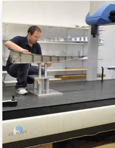
Inspecting Aircraft Structural Components with CMM, Aircraft Philipp, Germany
