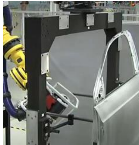
Car body component inspection, White Light System, SEAT, Spain
